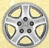
15x7-inch Ecco Cast Aluminum Available in the Ecco Wheel and Tire Group
