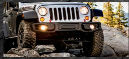
Battle the boulders with stamped steel skid plates that help protect Rubicon's beefy guts. Brawny Dana® 44 heavy-duty solid front and rear axles are standard fare. Rock-Trac® 4WD with a 4:1 low-gear ratio lets Rubicon overcome radical obstacles at low speeds for greater control, increasing the amount of torque pushed to the wheels. Electronic Front Sway Bar Disconnect permits an intimidating display of articulation. Removeable front bumper end caps provide maximum maneuverability.
