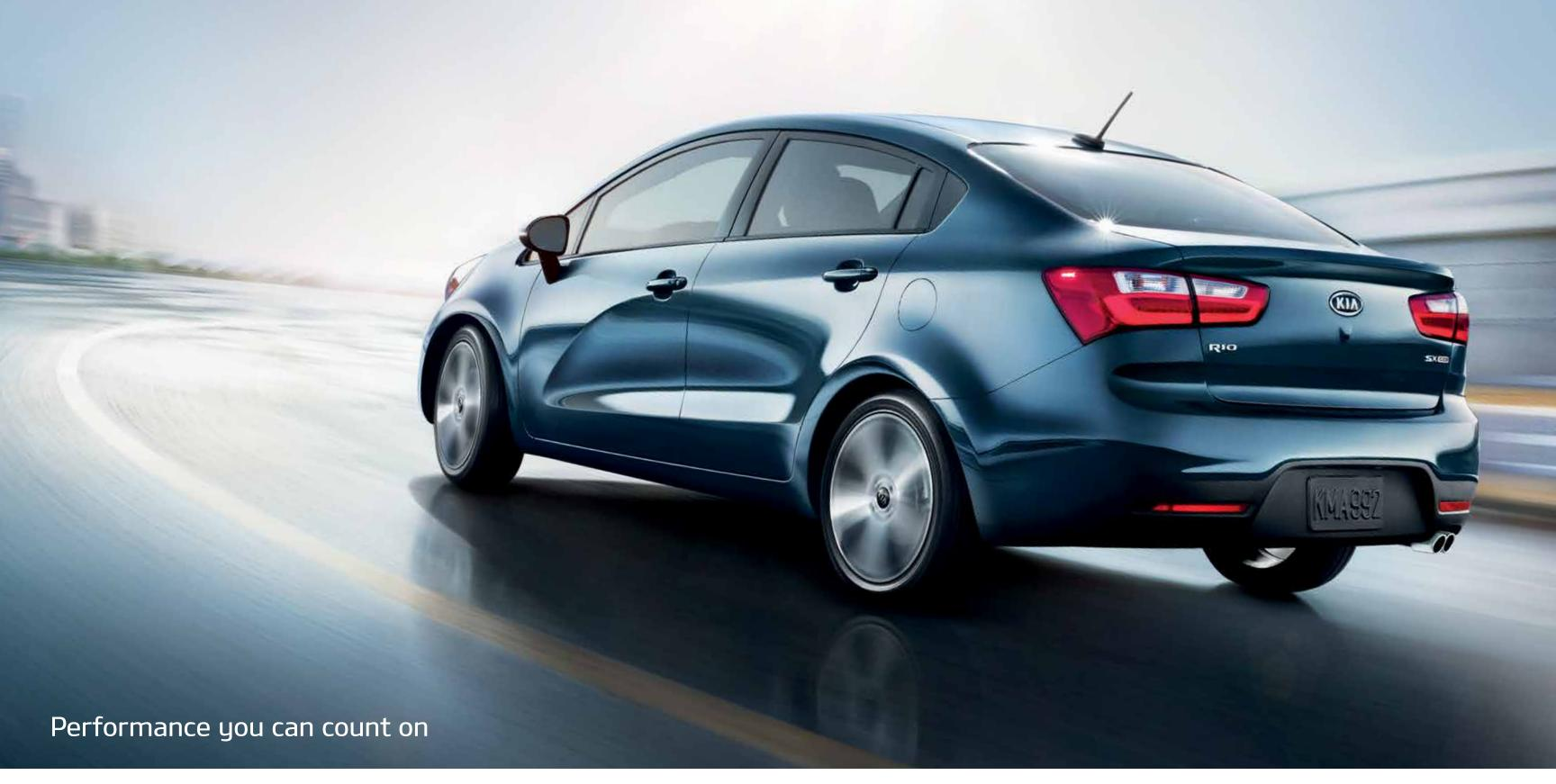
Rio delivers outstanding performance that puts the fun back into driving. It features a Gasoline Direct Injection (GDI) engine with 138 horsepower and an available smooth-shifting, six-speed automatic transmission.\* For increased agility and responsiveness, Rio SX features a sport-tuned suspension and 17-inch alloy wheels.
