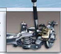
INSPIRING ROAD MANNERS. A fully independent suspension system—including MacPherson struts up front, an advanced multilink design in the rear, plus front and rear stabilizer bars—results in agile handling and exceptional ride comfort.
