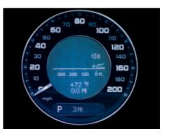
Available on the E63 AMG, this radar-based breakthrough monitors the vehicle ahead and adjusts your speed to help maintain a selected following distance.<sup>29</sup> If the vehicle ahead suddenly slows or abruptly stops and calculated closing speed indicates that you haven't taken appropriate braking action, the system illuminates a red light in the instrument cluster and sounds an alarm signal.<sup>30</sup> Ideal for long journeys, as there is less need to adjust the cruise control setting.
