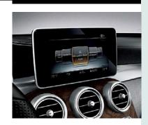
7" color screen and rotary central controller; or COMAND® with navigation, 8.4" screen and touchpad controller\*
