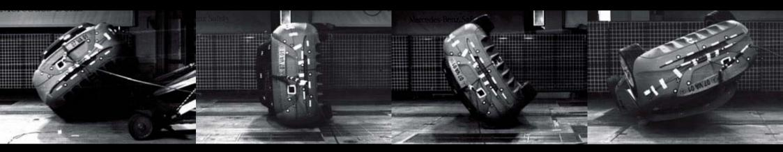
The SLR Roadster put to the test: the roll-over bars and the extremely rigid A-pillars provide an optimal level of protection for the occupants in the monocoque
