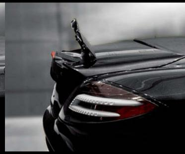
The AIRBRAKE in zero position
