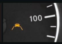
Lane Keeping Assist<sup>6</sup> provides the driver audible and visible warnings if the vehicle leaves its lane unintentionally. A camera in the windshield monitors the road ahead, detecting when you may veer away from lane markings.
