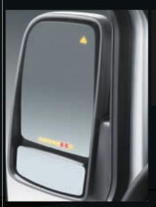
**Blind Spot Assist**<sup>5</sup> helps the driver avoid accidents by giving visible warnings when it detects vehicles in the blind spot.
