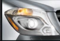
**Highbeam Assist** utilizes a camera located on the inside of the windshield to monitor traffic ahead. When activated, it controls the headlight main beam to provide the best possible road illumination.
