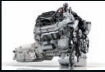
The optional 3.0-liter V6 turbo diesel engine is a proven powertrain that offers powerful acceleration, 325 lb-ft of torque combined with a smooth 5-speed transmission.
