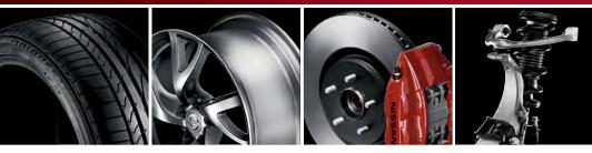
**Lightweight suspension components.** The lighter a suspension's components, the more quickly it can react to the driver and bumps in the road. Use of strong yet lightweight aluminum makes the  $Z^{\circledR}$  suspension extremely responsive. Its double-wishbone front and 4-link rear design helps to keep the tires vertical to the ground, maximizing their contact patches. Dual flow pass shocks enhance control. And super-light forged 19" alloy wheels are available for even quicker response.
