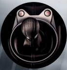
A world's first. Included on the Sport models, SynchroRev Match® technology - the first in any production car monitors the 6-speed manual's clutch pedal, shift lever, and vehicle speed. As you shift to a lower gear, the system will "blip" the throttle to the ideal engine rpm for a supremely smooth downshift as you let out the clutch. The system also works when upshifting to give you a smooth flow of power when accelerating.
