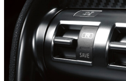
Transmission settings: R-Mode, Normal and Save
