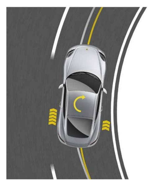
**Porsche Torque Vectoring (PTV)** PTV is an optional system for enhancing driving dynamics and stability. Operating in conjunction with a mechanical rear differential lock, it works by varying the amount of torque transmitted to the rear wheels.
