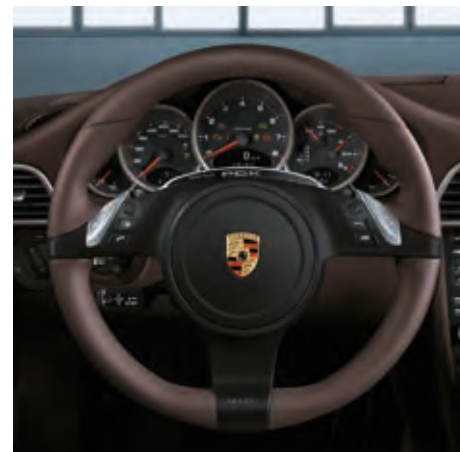
Three-spoke sports steering wheel with gearshift switches in conjunction with PDK and Sport Chrono Package Plus
