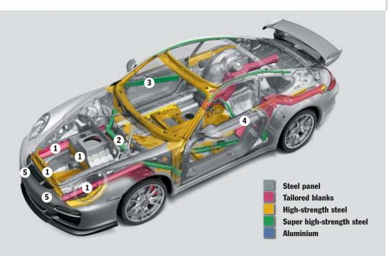
minor collision, a system of easily replaceable impact absorbers (5) prevents more serious damage.
