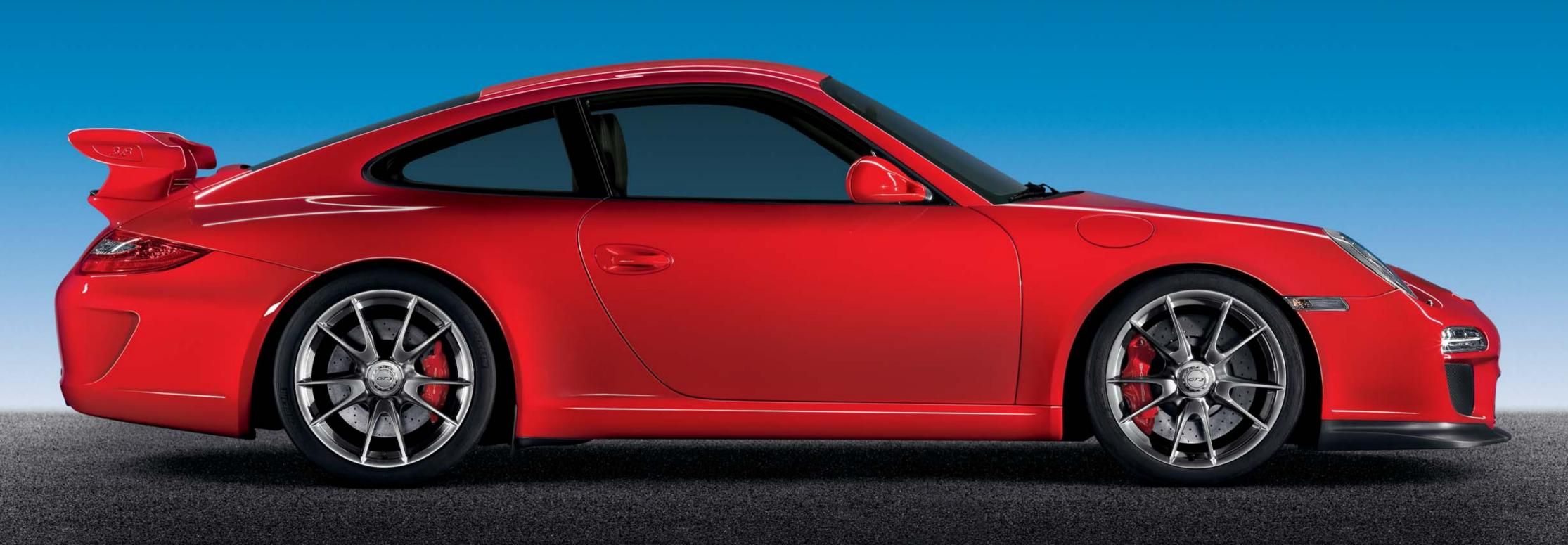
At the rear, distinctive LED lights are drawn right into the wing and taper outwards. Unmistakable just like the fixed bi-plane wing. This provides aerodynamic downforce and greater driving stability, even at the highest speeds. It is made from light-weight synthetic material and the angle of incidence on the upper wing profile can be adjusted for use on the racetrack. Embossed on the side plates of the rear wing: '3.8'. A
