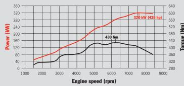
911 GT3: 430 Nm at 6.250 rpm, 320 kW (435 hp) at 7.600 rpm
