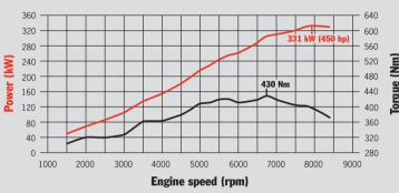
911 GT3 RS: 430 Nm at 6,750 rpm, 331 kW (450 hp) at 7,900 rpm
