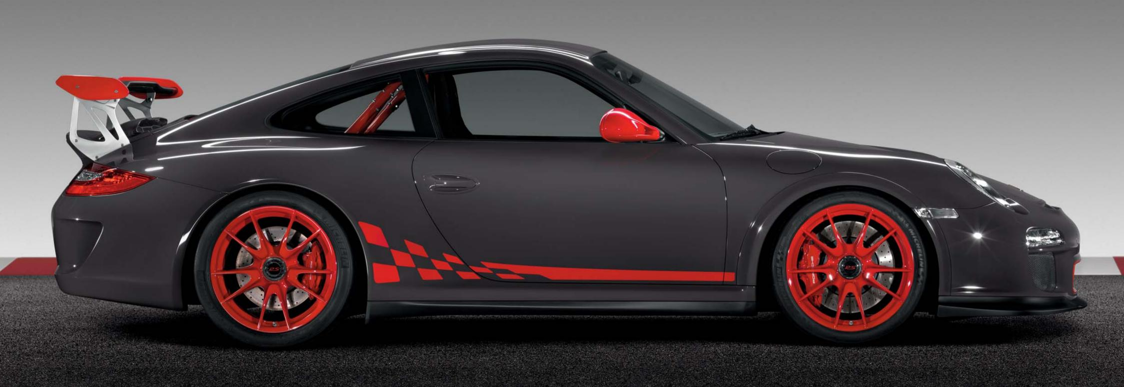
The engine lid with a 'GT3 RS' logo and the rear window are made from a lightweight synthetic material, as is the new rear middle section. A typical feature is the additional large air inlet on the engine cover (ram-air collector) for increased air intake and even better cooling.
