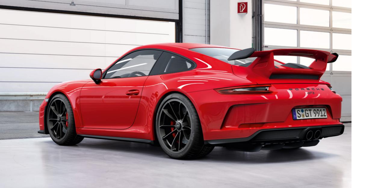
Broad is how the rear looks. And broad is also its stance on the road. That's because the 911 GT3 is an extra 44 mm (1.7 in) wider and sits approximately 25 mm (1 in) lower than the 911 Carrera. It's because the LED taillights are not only slim, they are now also shaped three dimensionally. It's because the central twin tailpipe of the sport exhaust system is a visual clue to the car's low center of gravity.
