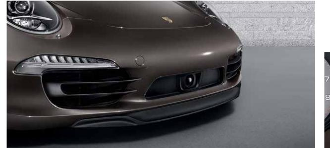
Radar sensor of Adaptive Cruise Control
