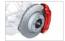
Standard brake system on the 911 Carrera S and Carrera 4S
