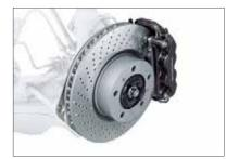
Standard brake system on the 911 Carrera and Carrera 4
