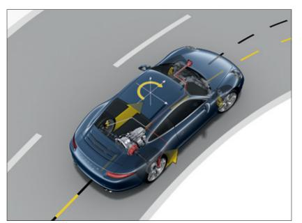
PTV in conjunction with the manual gearbox, or PTV Plus with Porsche Doppel-kupplung (PDK), are available as options for the 911 Carrera models and standard in the 911 Carrera S models. Both systems actively enhance vehicle dynamics and stability. Operating in conjunction with a mechanical (PTV) or electronic (PTV Plus) rear differential lock, they work by braking the rear wheels as the situation demands.
