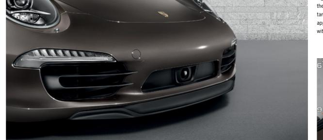
Radar sensor of adaptive cruise control
