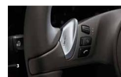
With the Sport button selected, the full advantages of the new version of PDK are brought into play: a more immediate response to throttle inputs; even shorter shift times; and swift, throttle-blip downshifts on overrun and when braking. Even the sound you hear from the exhaust is altered to elicit a more visceral response.
