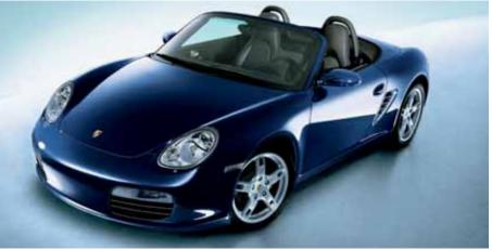
Passive safety features include full-size front airbags for driver and passenger as well as Porsche Side Impact Protection (POSIP see page 56). The POSIP package includes head and thorax airbags which are fully effective even when the hood is open.
