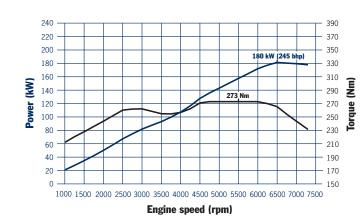
Boxster: 273 Nm between 4,600 and 6,000 rpm, 180 kW (245 bhp) at 6,500 rpm
