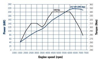
Boxster S: 340 Nm between 4,400 and 6,000 rpm, 217 kW (295 bhp) at 6,250 rpm
