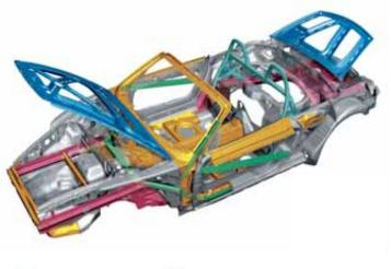
Sheet steel Tailored blanks High-strength steel Super high-strength steel Suner high-strength austenitic stainless stee element incorporated within the windscreen frame.
