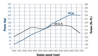
Boxster: 201 lb.-ft. at 4600-6000 rpm, 245 hp at 6500 rpm
