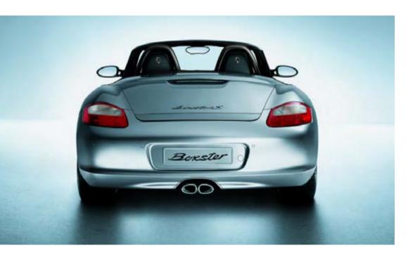
ParkAssist is an optional feature that is automatically enabled whenever you select reverse gear. Four sensors integrated into the rear bumper gauge distances to stationary objects, triggering a warning signal that increases
