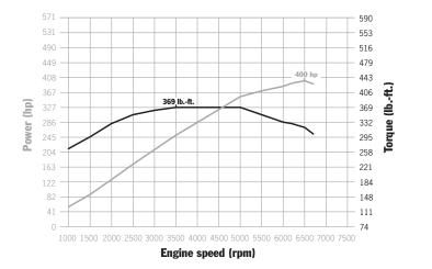
Cayenne S: 369 lb.-ft. at 3500 rpm, 400 horsepower at 6500 rpm
