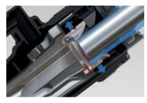
The blue outline shows the width of the diesel fuel nozzle, which is wider.
