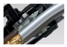
When the larger diesel fuel nozzle is inserted, the interlock opens to allow fueling.
