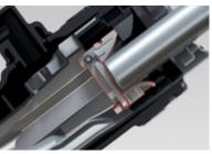
The smaller gasoline nozzle does not open the interlock.
