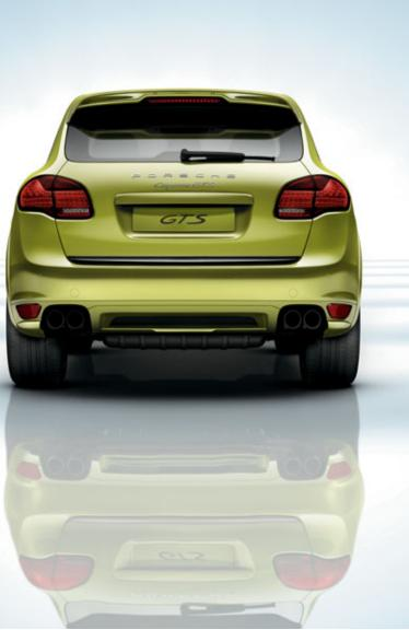
Cayenne GTS sport exhaust system with dual twin-tube tailpipes finished in matte black
