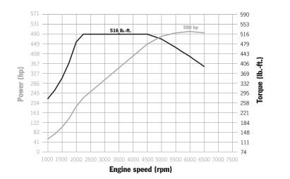
Cayenne Turbo: 516 lb.-ft. between 2250 and 4500 rpm, 500 horsepower at 6000 rpm
