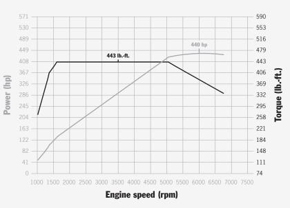
Cayenne GTS: 443 lb.-ft. between 1,600 and 5,000 rpm, 440 hp at 6,000 rpm
