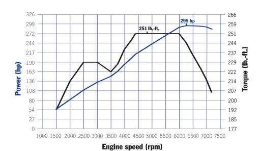
Cayman S: 251 lb.-ft. between 4400 and 6000 rpm, 295 horsepower at 6250 rpm
