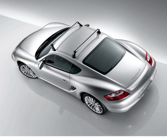
Roof Transport System (base load carrier)
