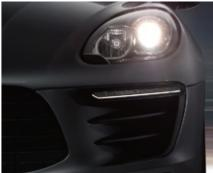
Dipped beam with halogen headlights
