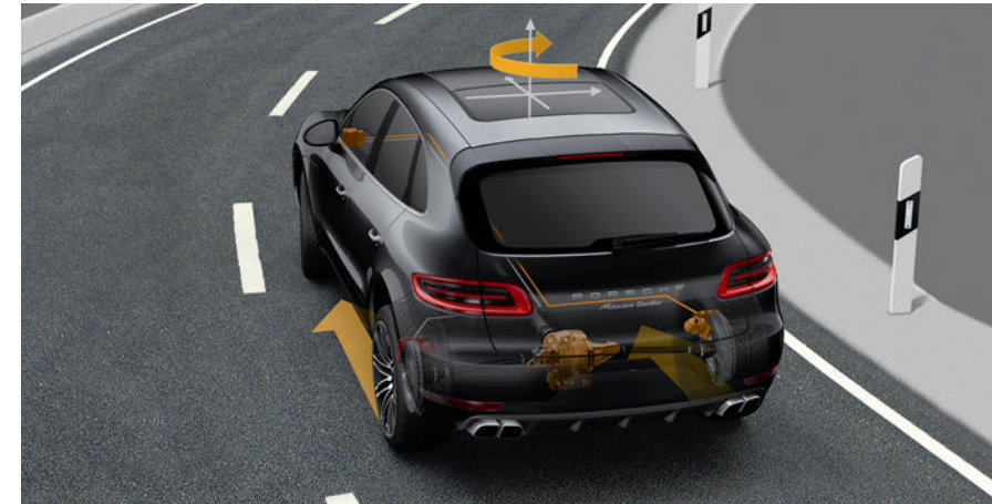
Porsche Torque Vectoring Plus (PTV Plus)
