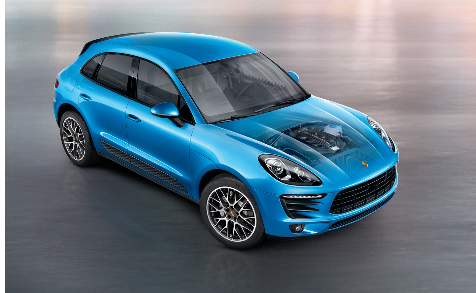
3.0-liter twin-turbo V6 engine
