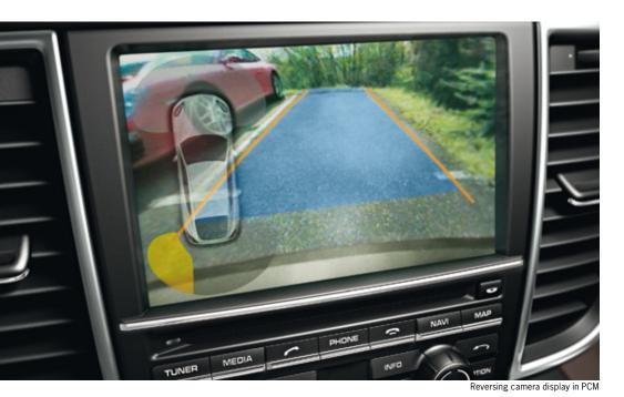
display screen which provides a graphical representation of the vehicle's proximity to obstacles.
