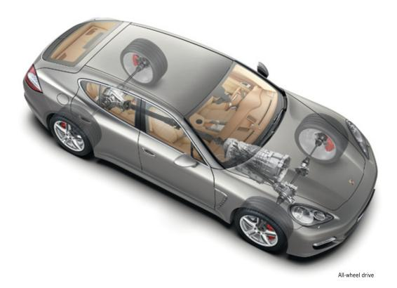
the multi-plate clutch. In addition, ASR reduces wheel slip. When cornering, the front wheels only ever receive as much drive force as is necessary to maintain optimum lateral stability.
