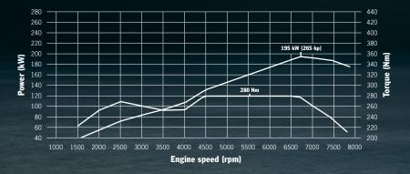
Boxster Black Edition: 195 kW (265 hp) at 6,700 rpm, 280 Nm between 4,500 and 6,500 rpm
