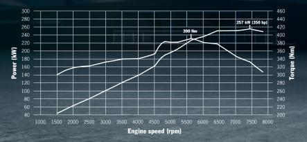
911 Carrera Black Edition models: 257 kW (350 hp) at 7,400 rpm, 390 Nm at 5,600 rpm
