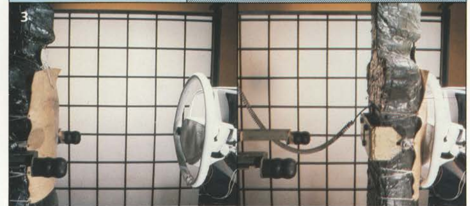
1: The fuel tank is located between the rear wheels, the safest location in case of collision. 2: The front coil springs are pivot-mounted to assure maximum control of the car even on uneven surfaces. 3: The Saab steering wheel will give way in the event of a serious collision, absorbing much of the driver's forward motion, in order to reduce possible injury.
