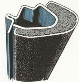
Roof pillars and windshield supports are covered with thick padding for occupant protection.
