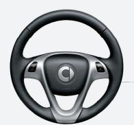
3-spoke leather sport steering wheel with cruise control or paddles for manual battery recuperation:
