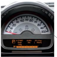
Trip computer: the easy-to-read multifunctional display shows current fuel consumption, mileage, trip information and more. Operated via the steering column control stalk. Available with cruise control package.
