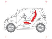
Safety seats with integrated seat belts and belt tensioners: the sheet steel structure with integrated headrests provides the smart fortwo's seats with a high level of mechanical stability. In a frontal impact, the seat belt tensioner reduces slack within milliseconds. The belt-force limiter then reduces the force again to minimize pressure on the driver and passenger.
