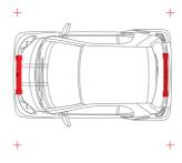
**Crash boxes:** steel deformation elements at the front and rear of the smart fortwo absorb energy from minor collisions at low speeds, ensuring that the tridion safety cell remains undamaged. Furthermore, a damaged crash box is simple to replace.
