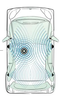
**New surround sound system:** for a new and improved audio experience. With subwoofer, eight-channel digital amplifier and tweeters, mid-range speakers and rear-fill loudspeakers. Available as an option on passion models only.
