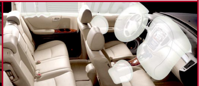
Driver and front passenger Advanced Airbag System. Available driver and front passenger seat-mounted side airbags and front- and second-row roll-sensing side curtain airbags. 1
