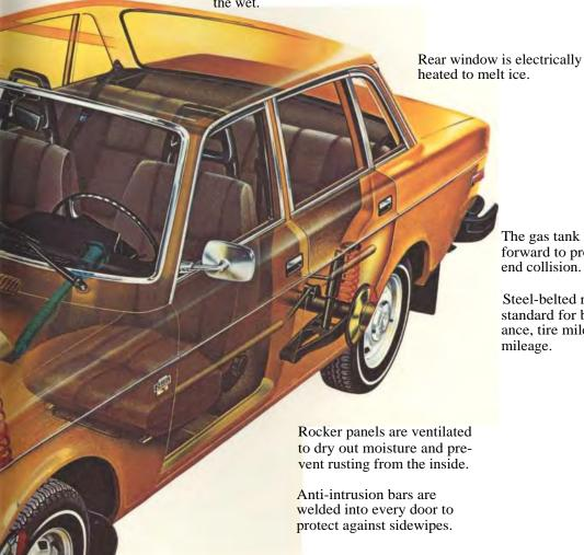
Rust susceptible panels, like those in the front-end, are made of galvanized steel.
