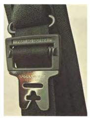
The Volvo self-adjusting safety belt is comfortable to wear. It unwinds from an inertia reel when you put it on. You'll find one for every corner passenger.
