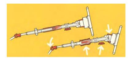
Four separate safety features are part of the steering column. Front left to right are: A breakaway joint and telescoping section - to prevent rearward displacement, and a slip joint and crumple zone - to absorb impact.
