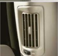
Adjustable air vents for the rear-seat passengers enhance comfort and help keep mist off the side windows.
