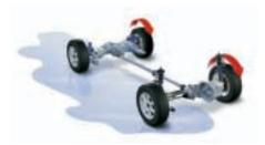
If one or both wheels on one side of the car spin, more power goes instantly to the wheels on the opposite side with the best traction.
