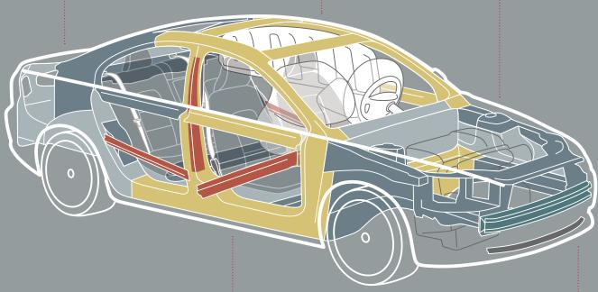
Incorporated in the front seats, the Whiplash Protection System (WHIPS) cradles the spine and neck in a controlled manner during and directly after a rearend collision of sufficient force. The robust safety cage uses various grades of high-strength and boron steel to distribute and absorb impact from all types of collisions to help protect the passenger compartment.
