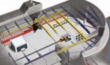
Within the center, our 850-ton barrier can be positioned and configured to replicate the dangers of countless real-life traffic situations. What's more, this is where collisions take place between a vehicle entering the center through the fixed tunnel and another entering from a pre-defined angle via the movable test track.
