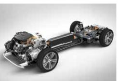
The S60 has been designed from the ground up with plug-in hybrid power in mind, so the batteries and electric motor are set lower in the chassis. This means more responsive, intuitive handling due to a lower center of gravity and more even weight distribution.
