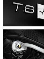
The front suspension is further stabilized by a Polestar Engineered strut bar. This contributes to even more precise, responsive steering characteristics at all speeds and more controlled handling through the curves.
