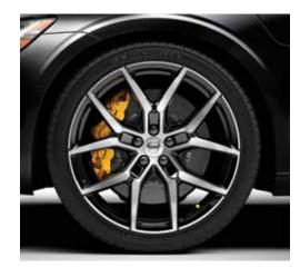
Reducing the unsprung weight by up to 15%, the Polestar Engineered 19" 5-Y Spoke Forged Wheels contribute to responsive driving characteristics and excellent road holding. Milled out of a solid block of aluminum, these wheels are of an exclusive design normally found on high-end performance cars and race cars.
