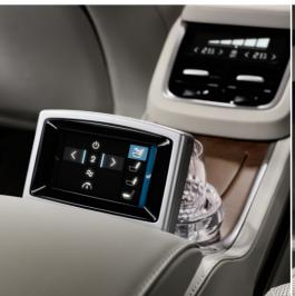
A pop-up touchscreen controls rear seat functions. When not in use it can easily be hidden from view.
