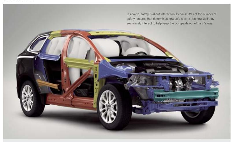
In a rear impact the rear deformation zones will help absorb crash energy. The fuel tank is designed to remain well protected in front of the rear axle. The head restraints help protect the neck and spine, and Volvo's unique Whiplash Protection System (WHIPS) cradles the front seat occupants in a controlled manner to help prevent whiplash injuries.
