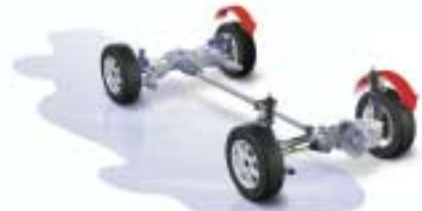
If one or both wheels spin on one side, more power goes instantly to the ones with the best traction.
