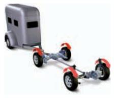
If you carry heavy loads, the rear wheels receive more power to maximize driving stability. Your Volvo XC70 can tow trailers weighing up to 3,300 lbs (1500 kg).
