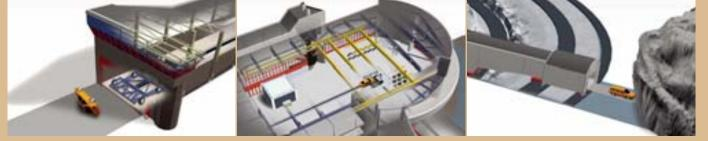
This fixed test tunnel is used for collision tests inside the center, and for rollover tests outdoors.
