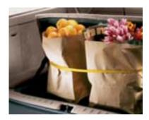
**GROCERY BAG HOLDER** Folds up from the cargo compartment floor and keeps your shopping bags securely in place. The bags are held in place by hooks or an elastic band. When not in use, it is hidden in the floor.
