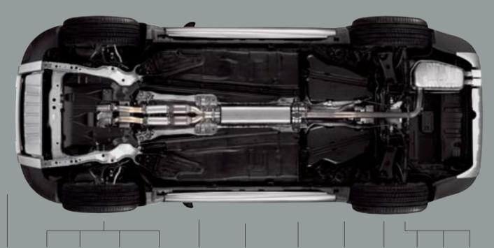
Anti-dive and anti-lift functions of the front suspension help maintain a stable attitude under hard braking or acceleration. Front suspension with McPherson spring struts. Stiffer antiroll bars help keep the car flat through hard turns. Firmer shocks improve body control and amplify road feedback.
