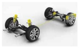
Choose the Off Road mode and the air suspension will raise the car by 40 millimeters. Hill Descent Control is activated at the same time: the car brakes for you on steep gradients – all you need to do is steer. The Off Road mode gets your XC90 to navigate challenging terrain – all you need to do is turn the elegant drive mode selector to the desired position.
