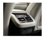
The 4 zone climate system can be controlled from the center touchscreen, or a graceful touch control panel at the end of the tunnel console.
