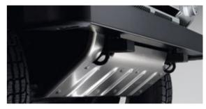
**Ribbed Aluminium Undershield** LR008247 Helps to provide under-engine protection when driving off-road. Undershield – Old Style (not shown) - STC50437 Aluminium blade with steel sub-structure.
