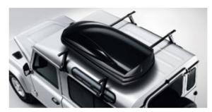
Luggage Box\* VPLVR0062 Opens from both sides. Lockable for security. External dimensions: 1,750mm long, 820mm wide, 450mm high. Volume 440 litres. Maximum payload 75kg†.
