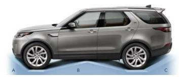
Ride Height Air suspension Coil suspension Approach Angle 34.0° 26.3°
