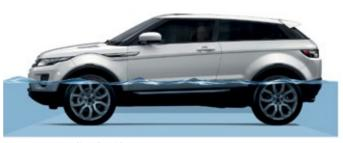
Wading Depth Maximum wading depth 19.7 inches (500mm)
