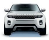
Obstacle Clearance Front axle clearance 8.4 inches (215mm) Rear axle clearance 9.5 inches (240mm)
