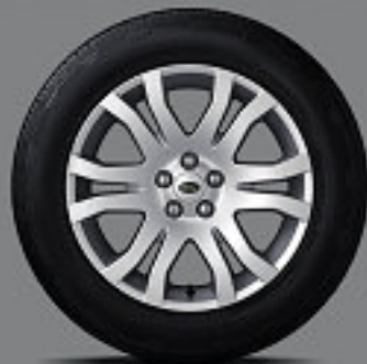
18 INCH 12-SPOKE ALLOYS – 235/60AT NO COST OPTION (APPROPRIATE SIZE FOR FITTING SNOWCHAINS)
