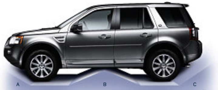
Off-road Geometry A Approach Angle B Ramp Break Over Angle C Departure Angle 29° 21.5° 32°
