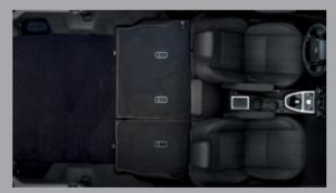
**LOADSPACE.** The versatile rear loadspace can be expanded by folding the 60:40 split rear seats to provide a flat load floor, and up to 58.9 cubic feet/1,670 liters of space. With 49 inches/1.25 meters between the wheel arches there's always room for more awkward loads.
