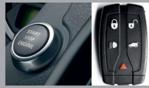
**START/STOP BUTTON AND REMOTE CONTROL.** In order to start the car the remote has to be docked into the fascia and the correct procedure followed using the Start/Stop button. The remote control includes the following functions: locking and unlocking of the doors and tailgate, a 30 second courtesy headlamp delay and activation of panic alarm.
