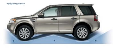
A Approach Angle 29° B Ramp Break Over Angle 21.5° C Departure Angle 32º
