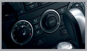
**CLIMATE CONTROL.** Standard air-conditioning system with dual-zone climate control, with pollen filter and humidity sensor maintaining fresh air in the cabin, keeping you and your passengers comfortable.
