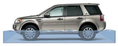
Wading Depth Maximum wading depth 19.7 inches/500mm
