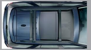
Raised Roof Rails and Cross Brace Kit\* Panoramic Sunroof vehicles LR007220 Vehicle height when fitted 72.0 inches/1,830mm. Crossbars not included.
