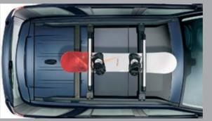
Ski and Snowboard Carrier\* LR006849 Carries four pairs of skis or two snowboards. Incorporates slider rails for easy loading. Lockable for security. Load capacity 79.4lbs/36kg\*\*.
