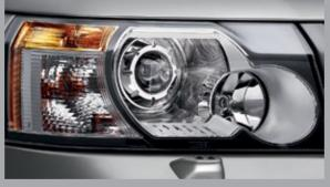
**HEADLAMPS.** Standard Halogen headlamps with impact-resistant polycarbonate lenses. Optional Adaptive Xenon projector lamps provide crisp blue-white light letting you see further and automatically swivel with the direction of travel to improve the view of the road ahead.
