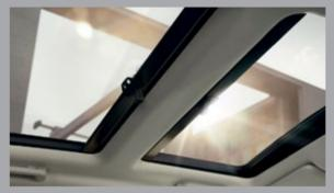
**PANORAMIC SUNROOF.** The standard panoramic sunroof – with a fixed rear section and electric tilting/sliding front section – adds to the feeling of lightness and airiness within the cabin. The glass is specially formulated to filter the sun's infrared rays, providing light without unpleasant heat. Both sections also include a convenient blind.
