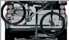
**Bike Carrier** LR008387 Fits to the Quick Release Tow Bar (LR019990). Holds four bikes (North America).
