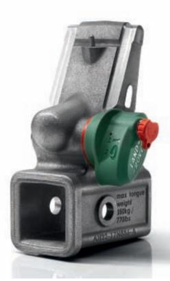
Quick Release Tow Hitch Receiver LR019990 Lockable for security. Easily removed. 1.9 inch Tow ball,
