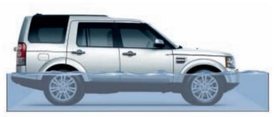
Wading Depth Maximum wading depth 27.56 inches/700mm, with air suspension raised Normal wading depth 23.62 inches/600mm
