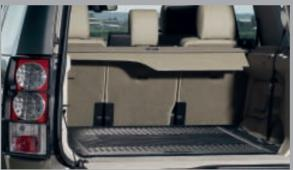
Loadspace Rubber Mat LR006401 Waterproof with retaining lip and non-slip surface.
