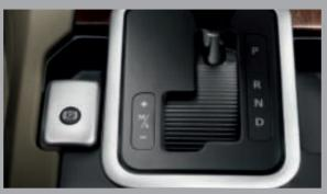
**ELECTRIC PARKING BRAKE (EPB).** A lever is located next to the gear selector to electrically apply and release the parking brakes on the rear wheels. A simple pull of the lever applies the brake manually and a press releases it. The parking brake will also release automatically upon driving away.
