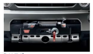
Electric Winch<sup>†</sup> VUB501471 9,500lbs/4,300kg maximum load capacity. Includes cover for protection when not in use. Plug-in remote control allows safe operation from up to 11.8ft/3.6 meters. Compatible with Protection Bar (VPLAP0022).
