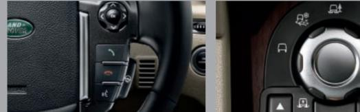
STEERING WHEEL CONTROLS. Steering wheel with ergonomically designed switch layout for driver information and remote audio controls. Cruise control is standard while telephone and heated steering wheel controls are optional and dependant on the vehicle derivative.
