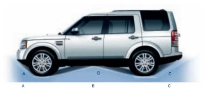
Approach Angle Standard ride height 32.2° Off-road ride height 37.2°, w/air suspension raised Ramp Break Over Angle Standard ride height 22.8° Off-road ride height 27.9°, w/air suspension raised Departure Angle Standard ride height 26.7° Off-road ride height 29.6°, w/full size spare option and air suspension raised
