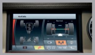
AIR SUSPENSION. Four-corner independent Air Suspension with variable ride height and electronic cross-linking for a constant level ride height. Ride height can be raised up 2.2 inches/55mm to clear obstacles or lowered by 1.9 inches/50mm for easy access and loading from standard ride height.
