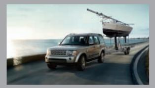
**TRAILER STABILITY ASSIST.** System helps make towing safer by detecting trailer oscillations and employing selective braking to help correct potentially dangerous situations.
