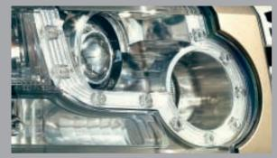
HIGH BEAM ASSIST (Optional) is designed to detect preceeding and approaching traffic and in a split second will automatically switch from high to low beam and back when the light source is out of range. The system is designed to distinguish between automotive and non-automotive light sources.
