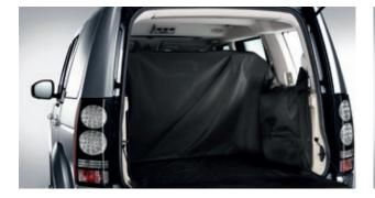
Flexible Loadspace Protector VPLAS0015 Heavy duty fabric helps protect loadspace up to window height. Also covers loadspace floor with second row seats folded. Includes heavy duty gloves.
