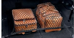
Loadspace Retention Net VUB503130 Utilizes loadspace tie-down points. Includes floor net and two ratchet straps. Strap length approximately 6.5 feet.
