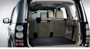
Loadspace Mat – Rubber LR006401 Waterproof with retaining lip and hard wearing surface.
